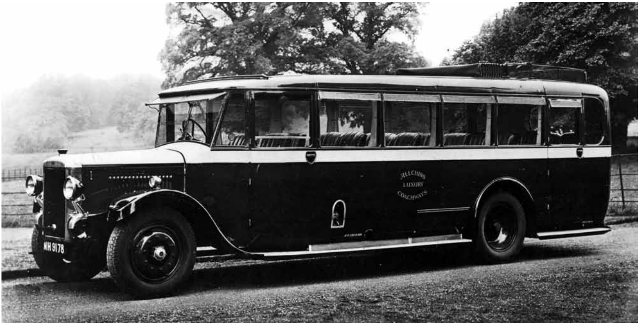
This handsome Daimler CF6 - NH 9178 - with sleek Hall Lewis coachwork and quiet six-cylinder sleeve valve petrol engine, must have literally glided along the roads of 1929 which were far less congested than today.
