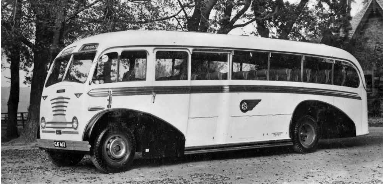
GJF 607 was a Dennis Lancet III with a full-fronted Yeates coach body seating thirty-seven passengers. Arriving in October 1950 it was the first new vehicle supplied to Seamarks by the Hamblin's Group. (Photo courtesy The Omnibus Society).
