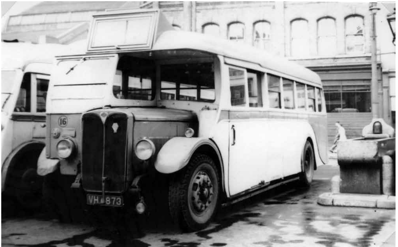
An illustration of one of the ex-Hanson's 1933 A.E.C. Regals with 1941 Burlingham thirty-five seat bus bodies acquired by Seamarks in January 1948. This bus was registered VH4873. (Photo courtesy J Bennett collection)
