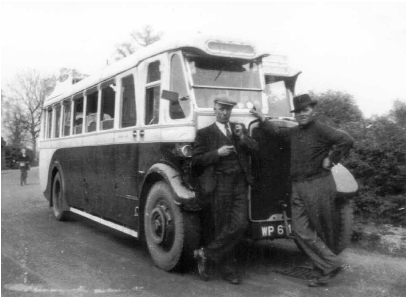
Leyland Lion WP 6113 with thirty-two seat Burlingham coachwork was acquired from Camplin of Donington circa 1942. This illustration shows it with Tom Head to the left and Frank Wiles to the right, probably in 1946.
