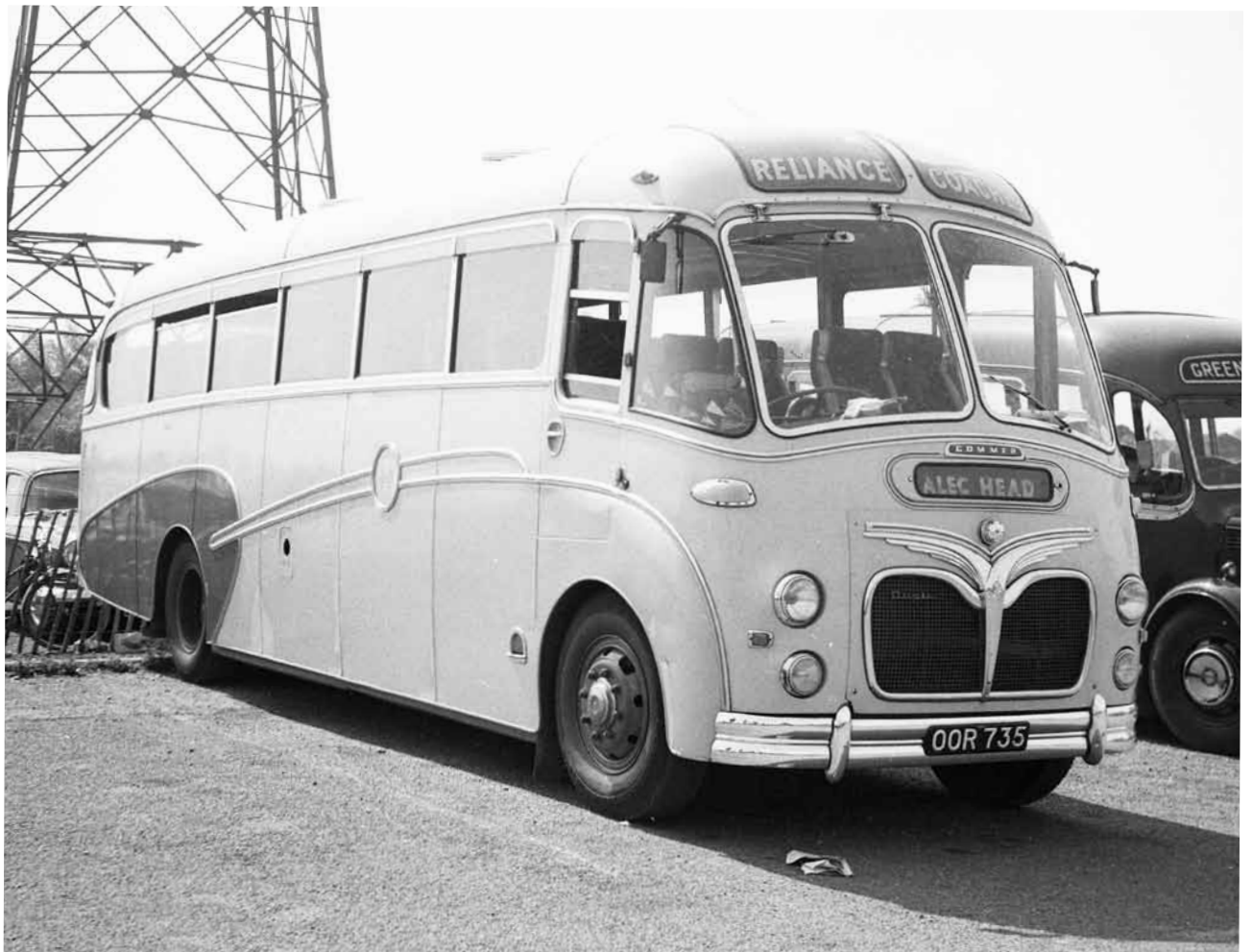
Reliance Coaches' premier vehicle in 1957 was OOR735, a Commer Avenger III with Duple Vega coachwork, replacing the 1951 Albion Victor on longer distance hires.
