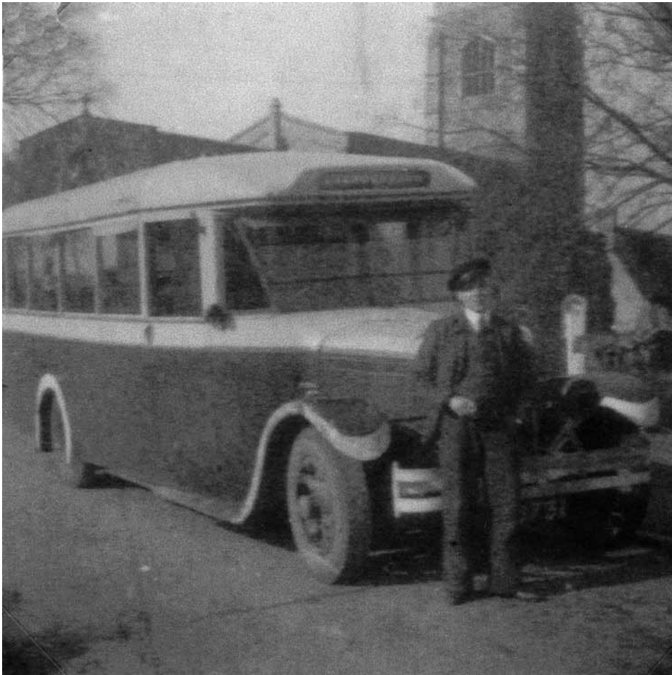
REO Pullman DO 8731 was bought by Tom Head from Teddy Shaw of Maxey in February 1942. It was photographed in the same year in the charge of driver Laurence Williamson and again sports war-time Hartley headlight masks and white tipped mudguards (Photo courtesy H Saville)
