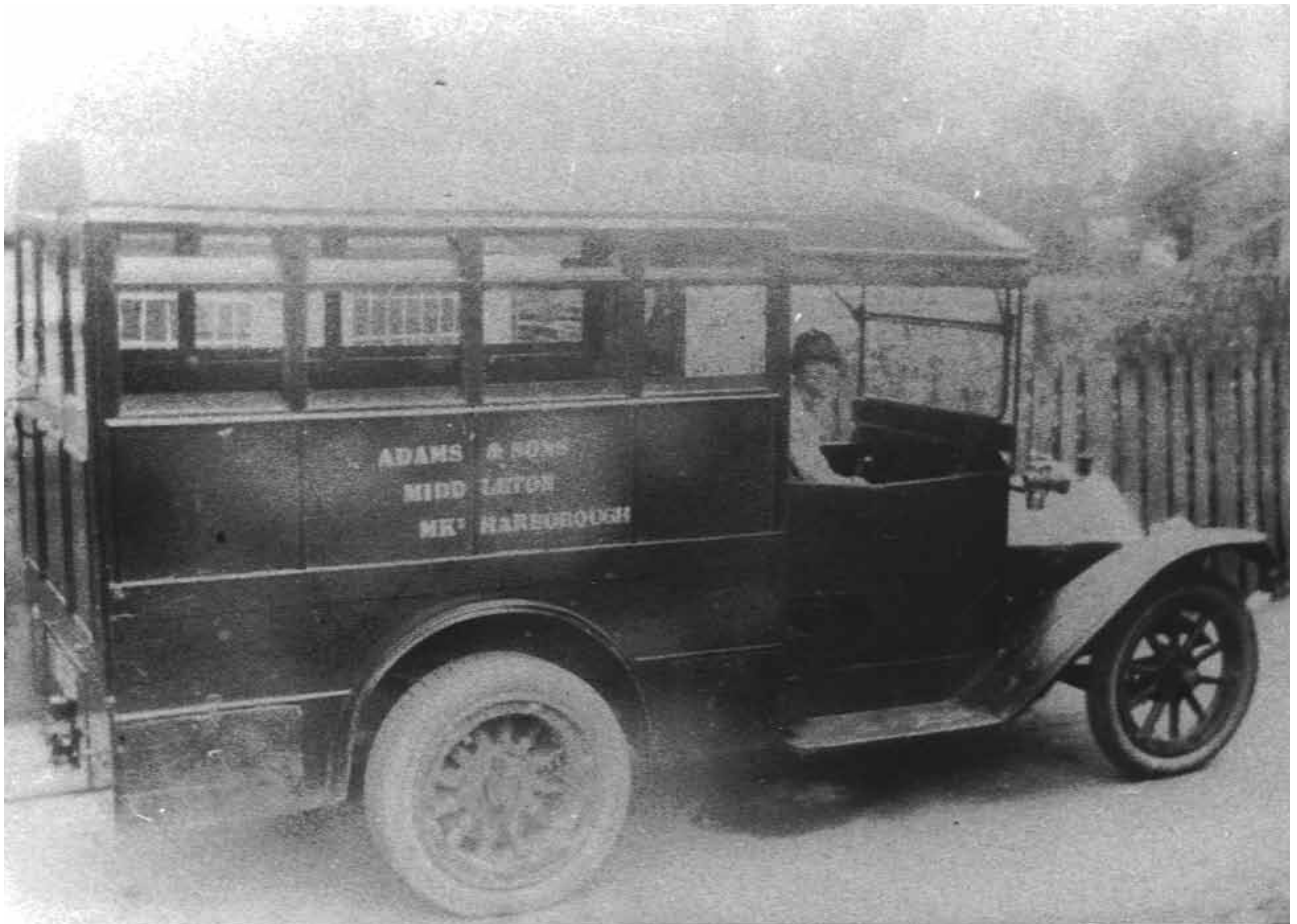
One of Alfred Adams Ford T buses photographed in the early 1920s after having been fitted with pneumatic tyres to the rear wheels. Hilda Adams occupies the driver's seat.
