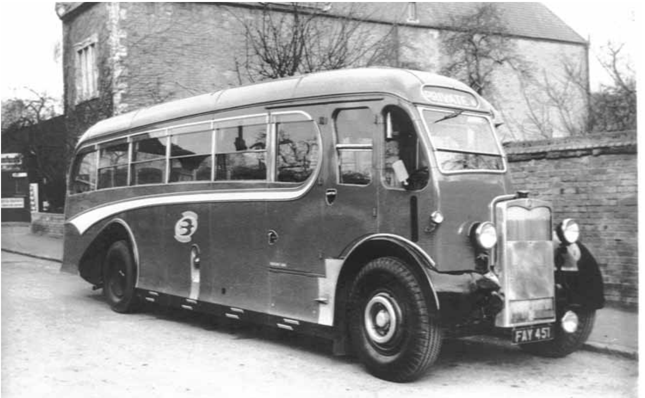
FAY 451 was an attractively proportioned Crossley with Burlingham thirty-three seat coach body on which the Adams' blue bird motif can easily be seen.
