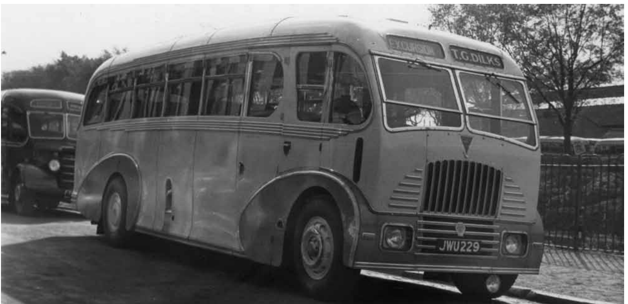
JWU 229 comprised an A.E.C. Regal III chassis with a full-fronted Burlingham body seating thirty-three passengers. Gerry Dilks ran it for about two-and-a-half years. (Photo courtesy D M Bailey)
