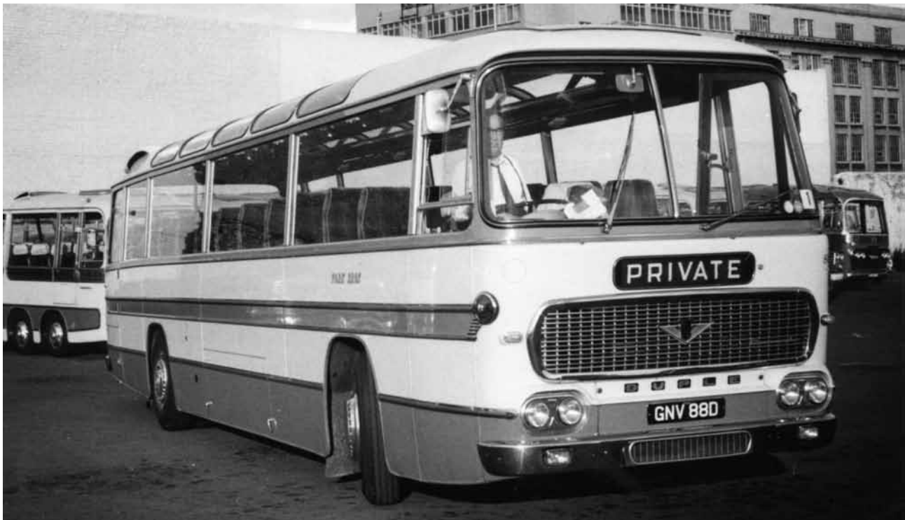
Another second-hand purchase was GNV 88D which can be seen here at Victoria Coach Station, London whilst with its original owner, York Bros. of Northampton. It is an A.E.C. Reliance 590 with Duple Northern Commander fifty-one seat coachwork.
