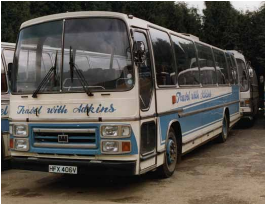
This Ford R1114 registered HFX 406V carried a Plaxton Supreme IV fifty-three seat body.
