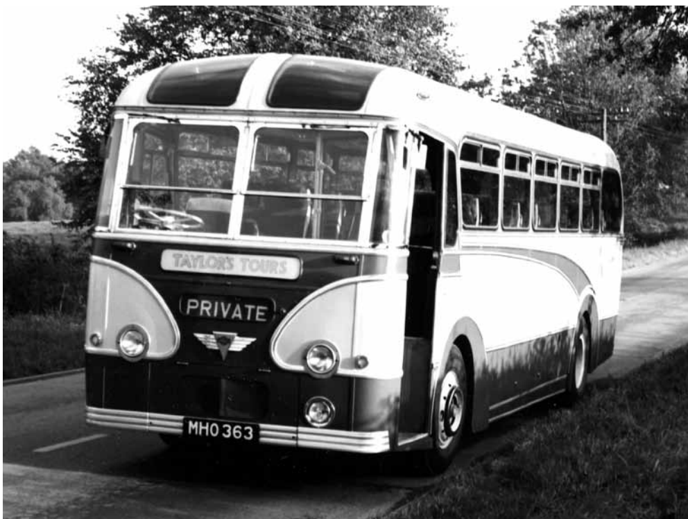
Mann Egerton built an attractive coach body for MHO 363, an A.E.C. Reliance that joined Taylor's fleet in May 1956. (Photo courtesy W Hadley)
