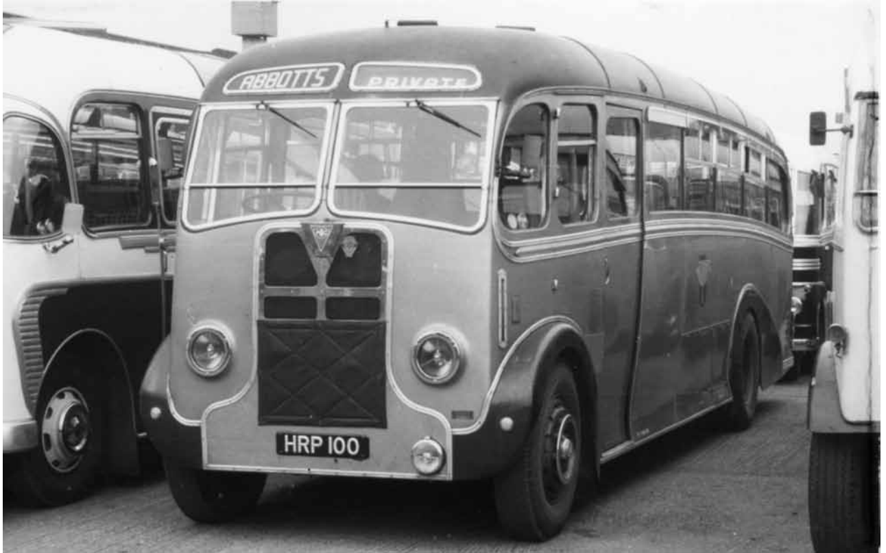
The nearside of the fully-fronted Whitson bodied A.E.C. Regal III registered HRP 100 can be observed in this illustration.
