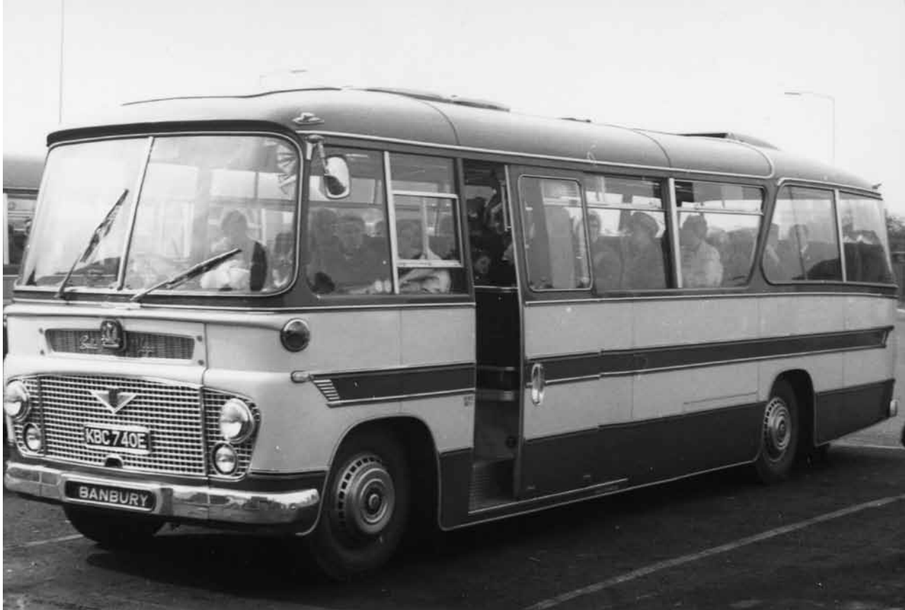
The last new coach to be acquired by George Owen was KBC 740E which was a Duple Bella Vega forty-one seat Bedford SB5. (Photo courtesy R H G Simpson).
