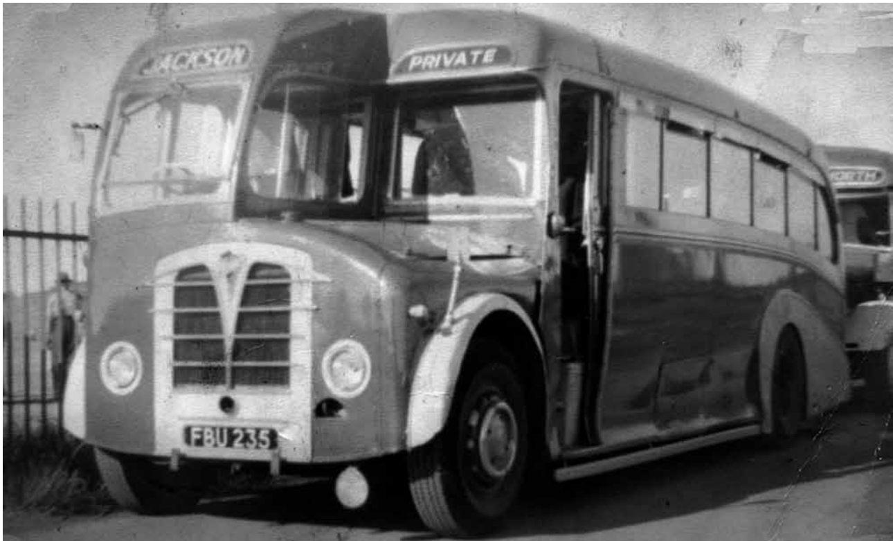
This illustration shows the Foden PSVC6 from the nearside. Jackson's name can be seen in the offside display aperture and no mention of Roydon Motor appears on the coach.
