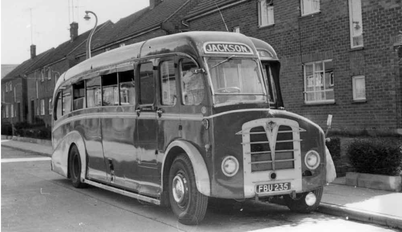
An offside view of FBU 235, the immaculate Bellhouse-Hartwell bodied Foden coach with which Don Jackson commenced business. (Photo courtesy M A Sutcliffe)
