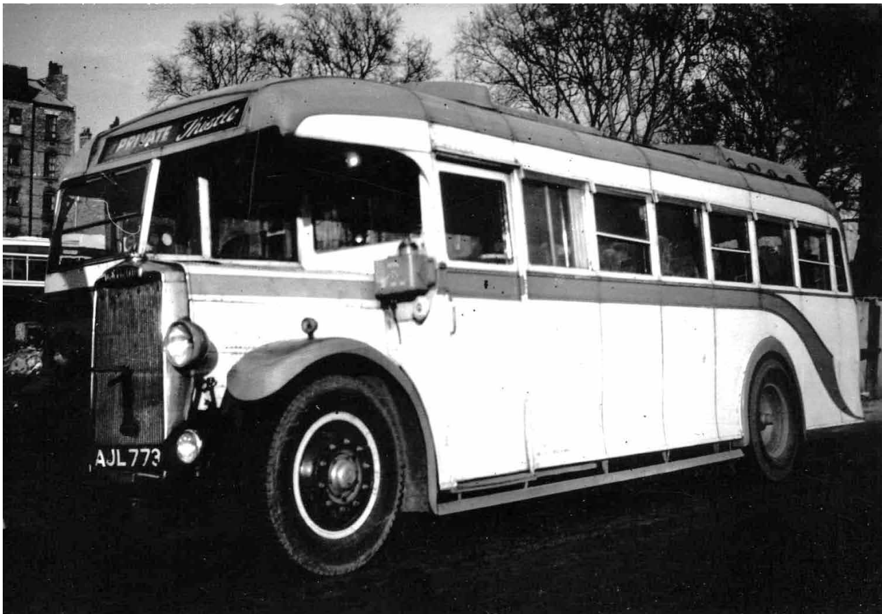
AJL 773 was a Leyland Tiger TS2 rebuilt in 1947 and mounted with an Alexander thirty-two seat body. Messrs Graveling and Wootton acquired it in October 1948.
