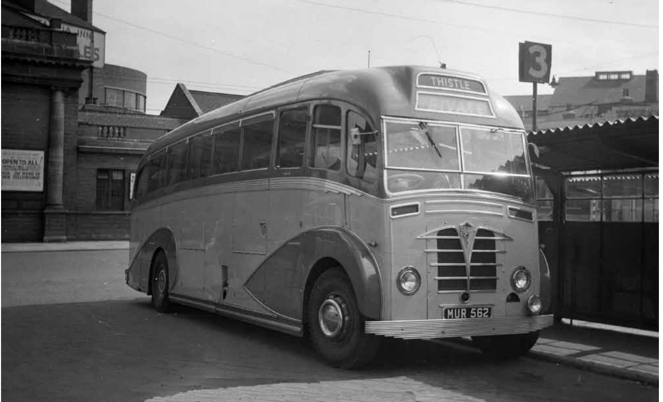
Thistle's Foden PVFE6 registered MUR 562 carrying a thirty-nine seat body by Windover. The livery of Thistle coaches was white and black. (Photo courtesy R Marshall).
