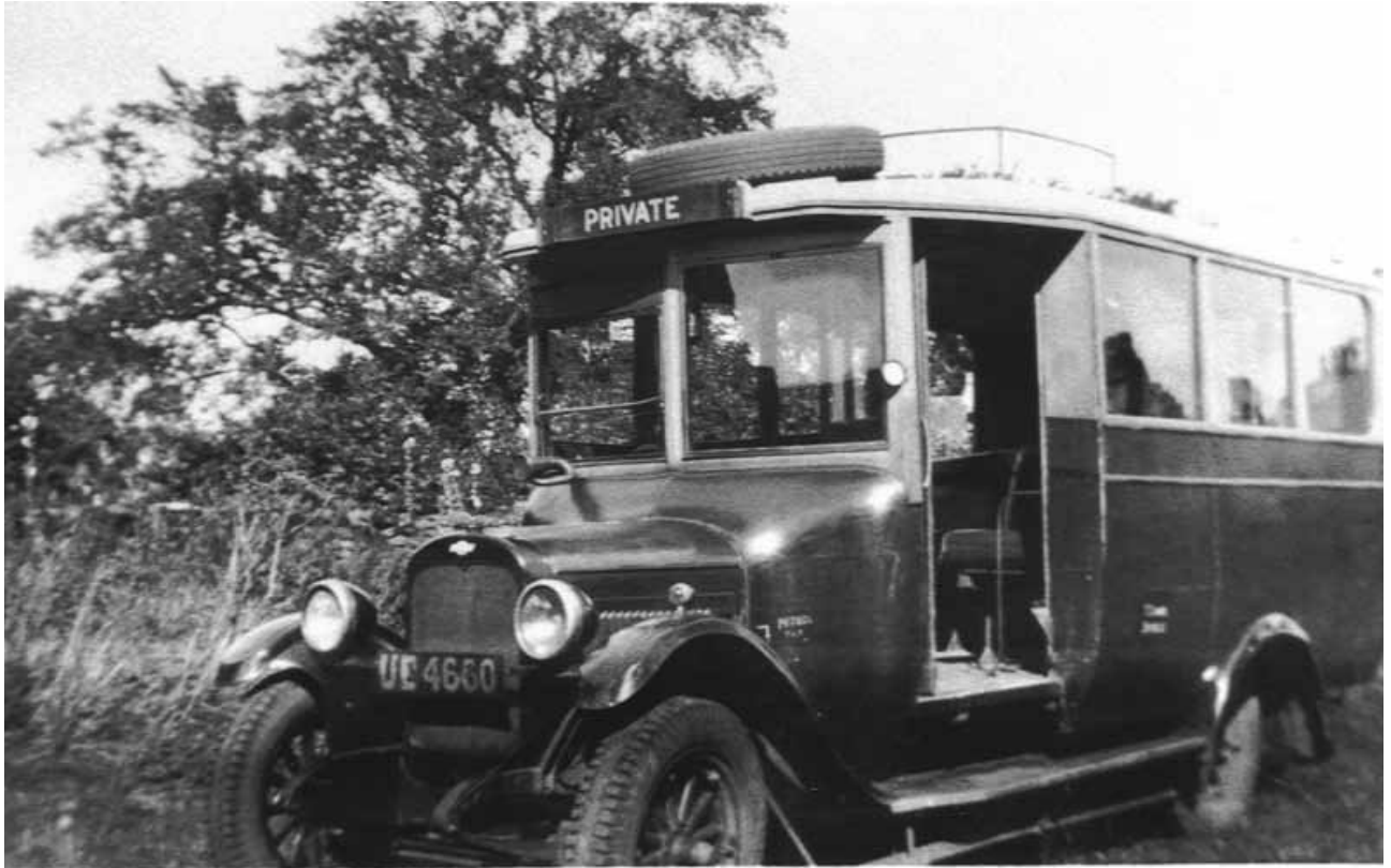
Thomas Lamb's Chevrolet registered UE4660. Note the luggage rack and roof-mounted spare wheel.
