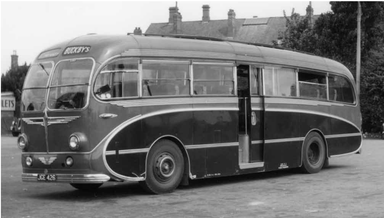
Burlingham Seagull bodied coaches were a popular choice of operators in the 1950s and this example is mounted on an A.E.C. Regal IV chassis and registered JGE 426. Jim Adams bought it second-hand in 1957.
