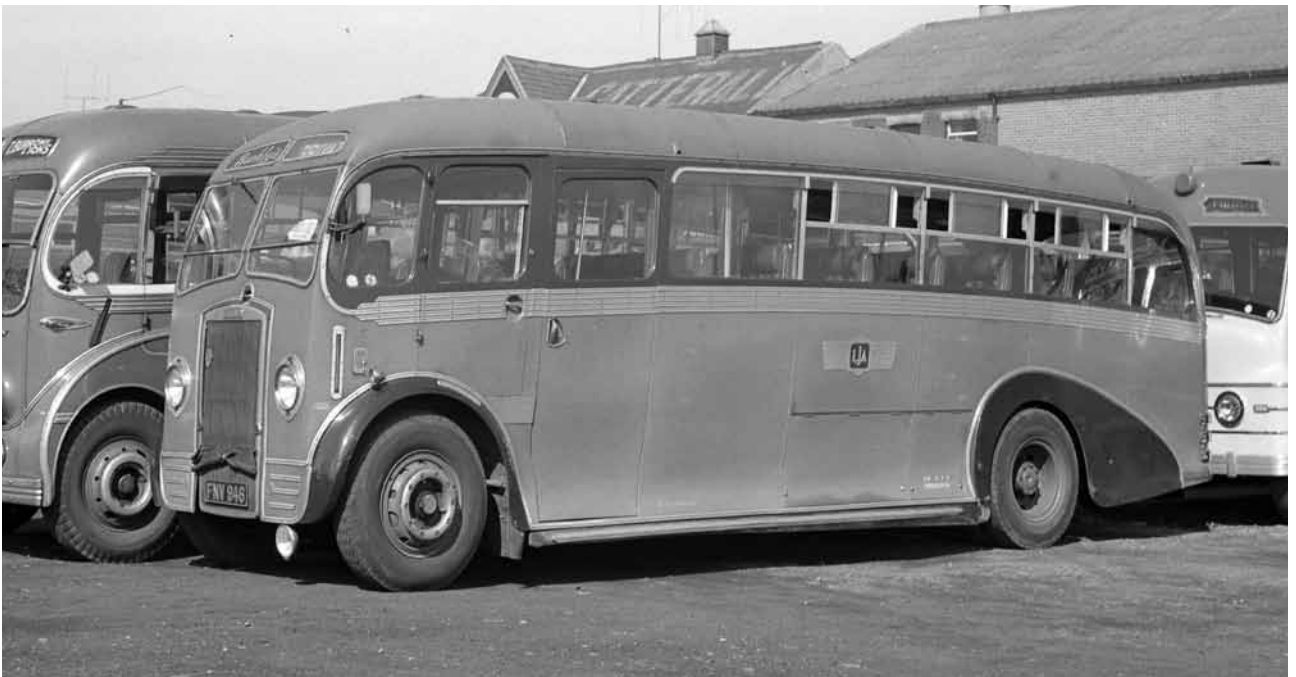
Not the sharpest of photographs but this illustration depicts FNV 946, a Leyland Tiger PS2/5 with fully-fronted Whitson body. The "L J A" monogram can be seen on the side of the coach.
