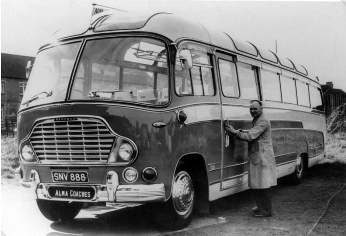
The petrol engined Bedford SB3 - SNV 888 - with Duple Vega coachwork was photographed when new in January 1959, its orange and cream paintwork gleaming in the winter sunshine. Rollie Walker entered SNV 888 in the 1959 Brighton Coach Rally.
