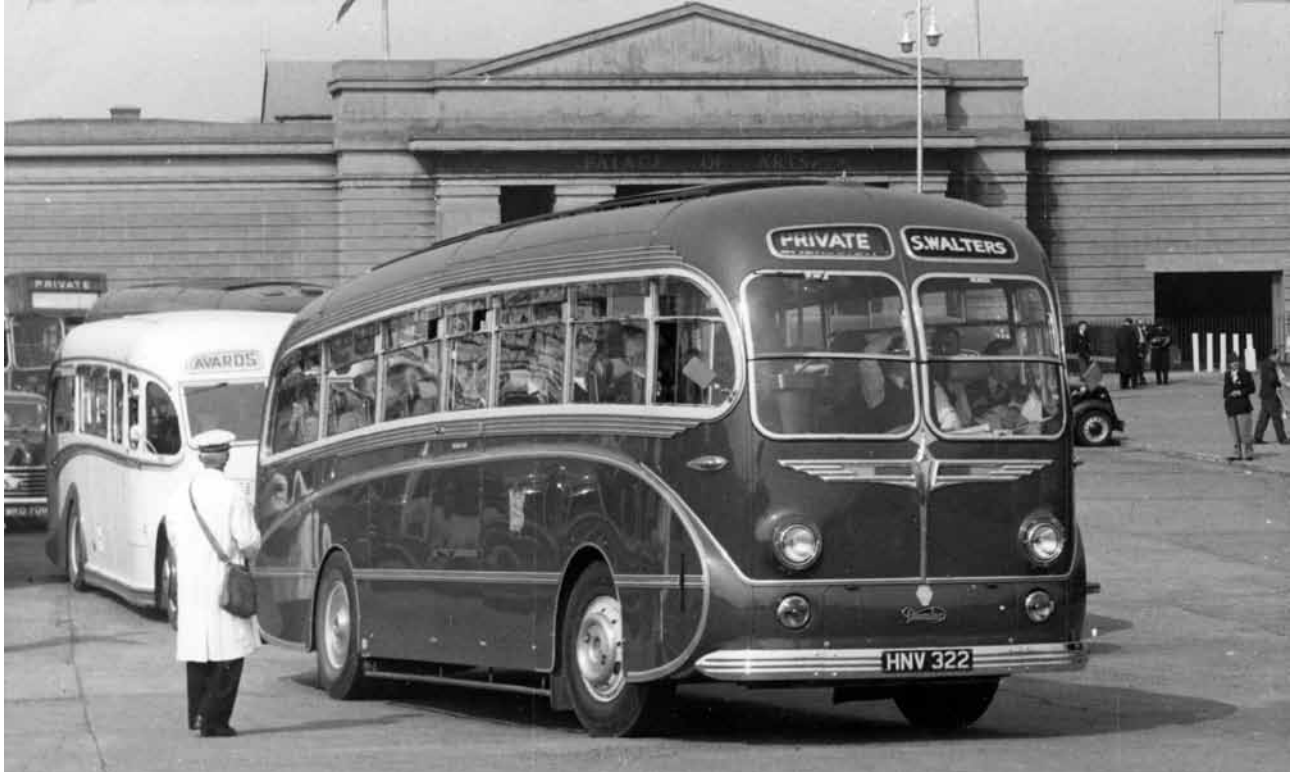
Sam Walters' attractive Burlingham bodied Daimler D650HS registered HNV 322 can be seen in this illustration. (Photo courtesy ATPH/Hustwitt)
