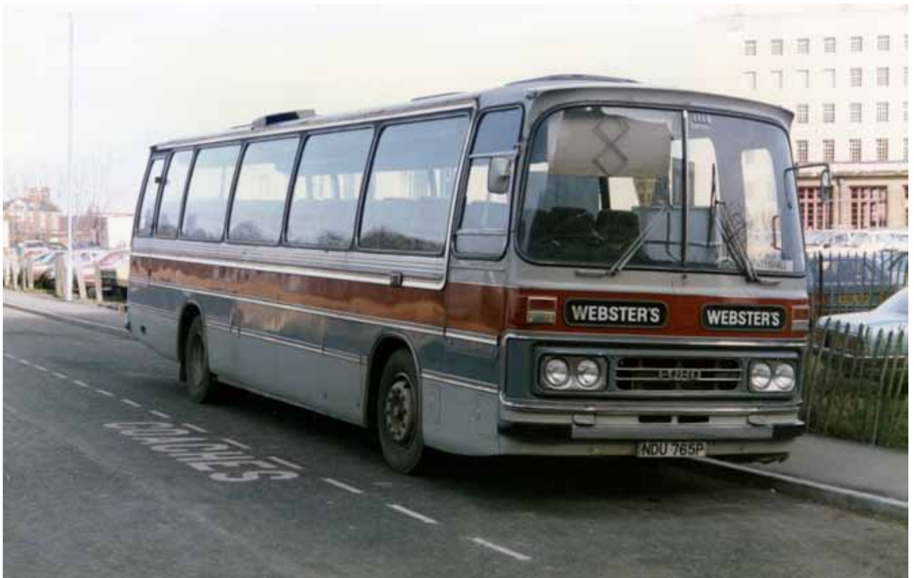
Being in sound condition, NDU 765P was repainted in Webster's fleet colours of two-tone grey and red for use on local service work. It was a Ford R1114 with 53-seat Duple Dominant body.
