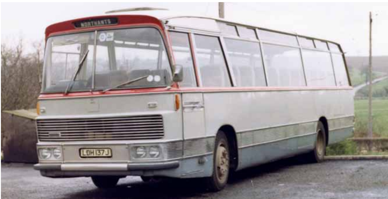
LDH 137J was a regular performer on the local stage carriage services after acquisition by Webster's in 1978. It was a Duple Viceroy bodied Ford R226 with a 53 seat capacity.
