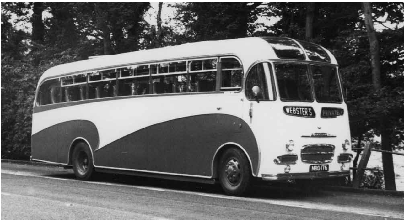
NBD 176 was a Commer Avenger II demonstrator new in 1954 with 41-seat Whitson coachwork that was bought by Harry Webster in March 1956. (Photo courtesy DM Bailey)
