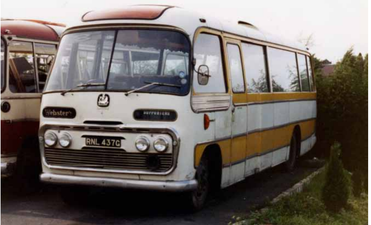
RNL 437G enjoyed only two years with Webster's, operating contracts from 1979 to 1981. Its Plaxton Embassy body was based on a Bedford SB5 chassis.
