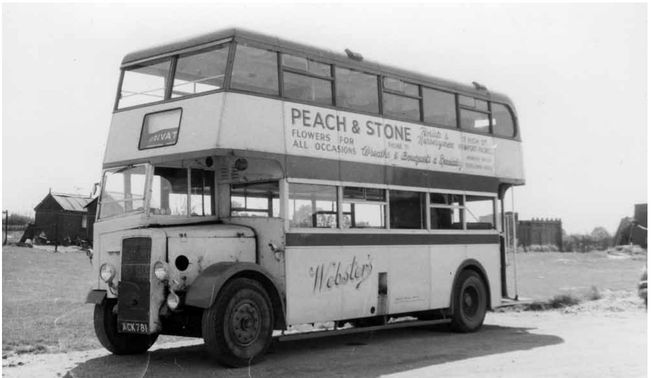
Harry Webster's first double-decker was this Daimler CWA6 with Brush 53-seat bodywork and registered ACK 781, purchased from Wesley of Stoke Goldington for school contract work. (Photo courtesy D M Bailey)
