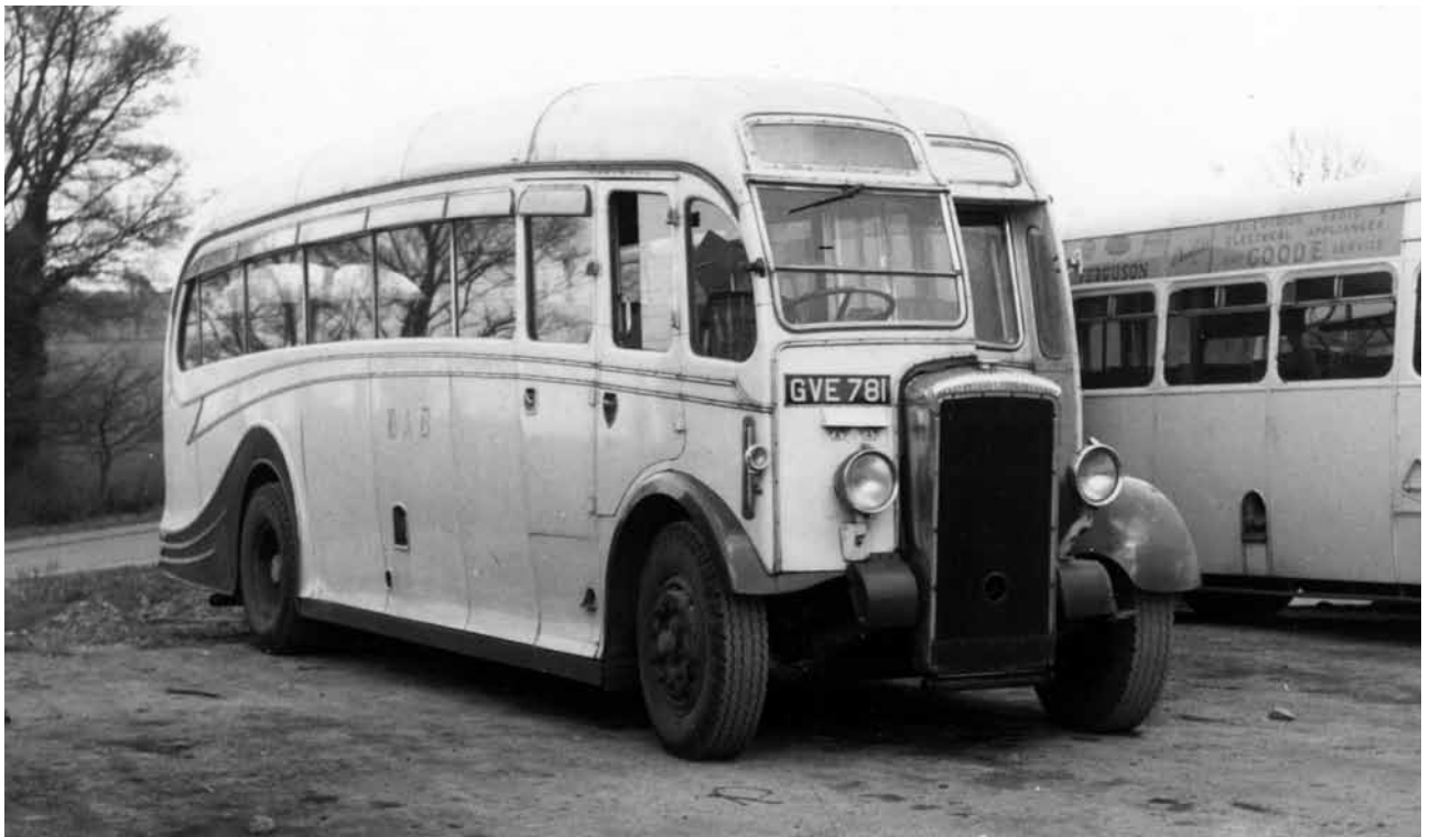
Harrington bodywork again features in this photograph but this time on a Daimler CVD6 chassis. GVE 781 was another former Burwell & District coach.
