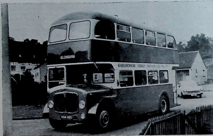
AEC Regent V HSN485 of Garelochhead Coach Services Ltd. This was new in 1958 and has a highbridge 65-seat body by Walter Alexander & Co. (Coachbuilders) Ltd. (Block by courtesy of "Passenger Transport").
