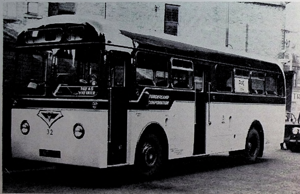
The first new bus to enter service in Sunderland since a recent announcement that future buses would be more comfortable and attractive is No. 32 (PGR332), an AEC Reliance with Park Royal group body attributed to Roe's. Although the chassis is an orthodox Reliance with synchromesh gearbox and the body design is also of orthodox p.a.y.e. practice, 32 nevertheless marks the most complete break from tradition ever found in one particular vehicle for Sunderland Transport and is much sought after on the routes on which it is operating. It is in its colour specification that 32 is outstanding. Externally it is painted cream below and green above the lower band of a double waist band in contrast to the previous livery of green with cream relief. Inside, the front-entrance centre-exit body has 41 tubular-framed service-coach seats upholstered in LTE Routemaster pattern moquette, with all trimming below the waist rail of red leather; the radiused metal window frames are stove enamelled primrose, and the Darvic plastic ceiling panels are in a pastel shade of blue with slightly darker blue stringers. A blue Cronaprest continuous bell strip is fitted above the windows on each side, and the interior specification is completed with heaters, fluorescent lights behind attractive plastic shades, full-length stainless-steel handrails and a compartment for luggage or push-chairs immediately behind the exit. A drop-frame at the front allows a lower and wider platform beside the driver with another step into the saloon. (Block by courtesy of the "Sunderland Echo")
